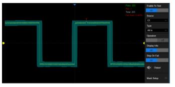
The SDS5000X utilizes a hardware-based Mask Test function, performing up to 18,000 Pass / Fail decisions each second. It is easy to generate user-defined test templates in order to provide trace mask comparisons, making it suitable for long-term signal monitoring or automated production line testing
